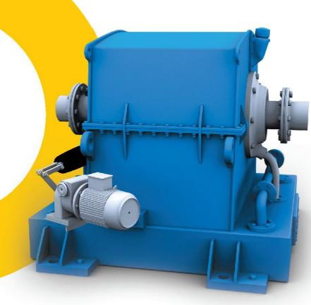
FLUIDOMAT -SC is a variable speed fluid coupling providing stepless speed variation in a wide range when connected to fixed speed electric motor. The speed variation is obtained by varying the oil filling in coupling through a sliding scoop tube when in operation.
