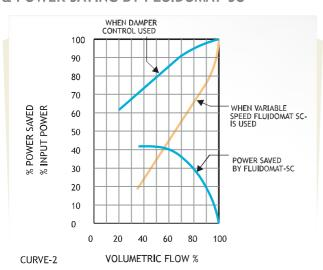
Curve 2 shows the typical example of power saved at different discharge values when Fluidomat SC is used. The power saving can be in the range of 10-40% depending on operation and flow requirements.
