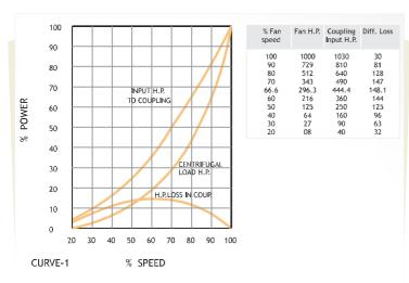
The curve 1 Shows the power required by a centrifugal machine at different speeds. In the same figure the power required by the system is shown if Fluidomat SC is used for speed variations. Fluidomat SC is an ideal equipment for speed variations of centrifugal machines & thus discharge control. Slip power losses in the coupling are also shown in the characteristic curve.
